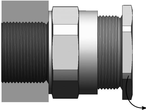
5. Pass the cable through the gland to the desired position, then tighten the seal nut by hand until resistance is felt (when the seal contacts the cable). Tighten with a spanner one further turn.
